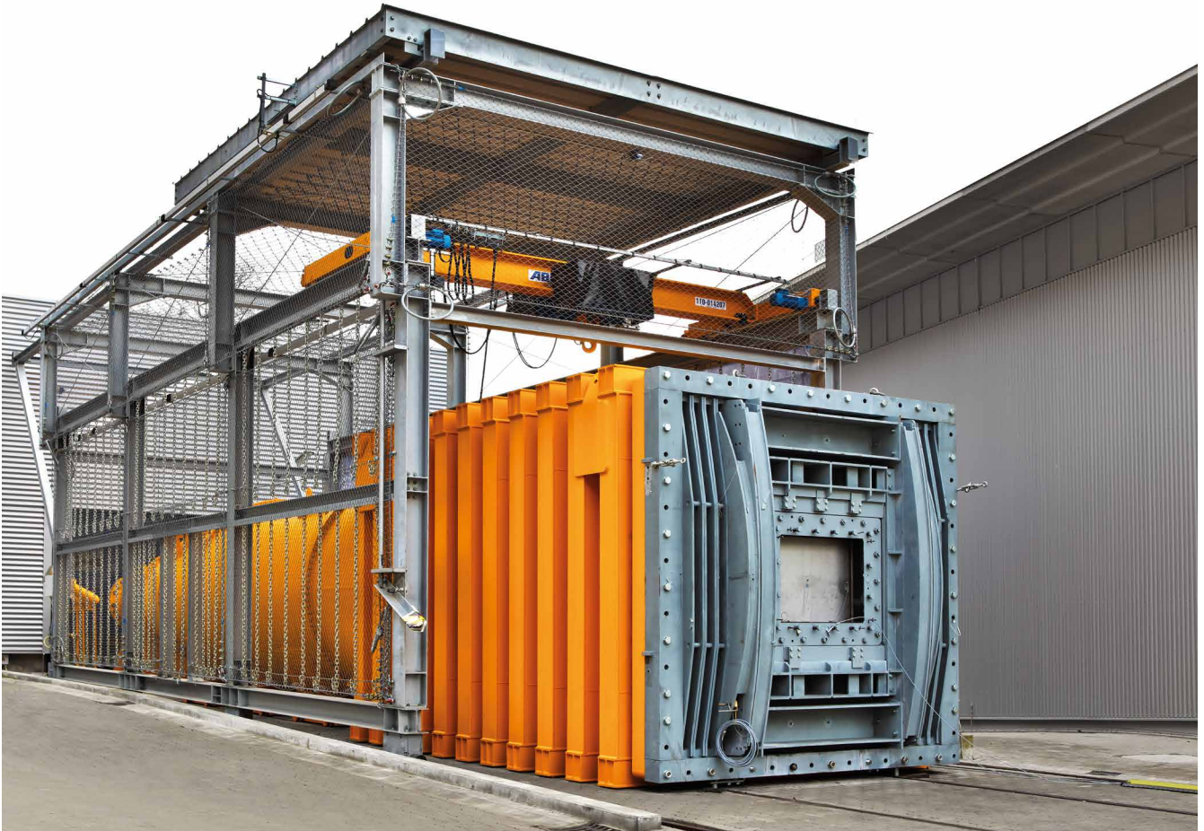
The shock-tube facility BlastStar at Fraunhofer EMI can be used to simulate shock wave loads resulting from explosives and gas explosions. The knowledge gained is used to optimize the materials and structures in use.
