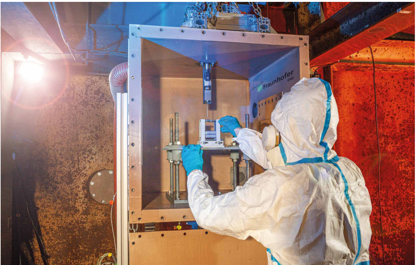
Top: the new TEVLIB laboratory for research into the failure of large lithium-ion batteries at EMI Efringen-Kirchen. Bottom: test chamber for battery failure investigations by means of in-situ X-ray technology.
